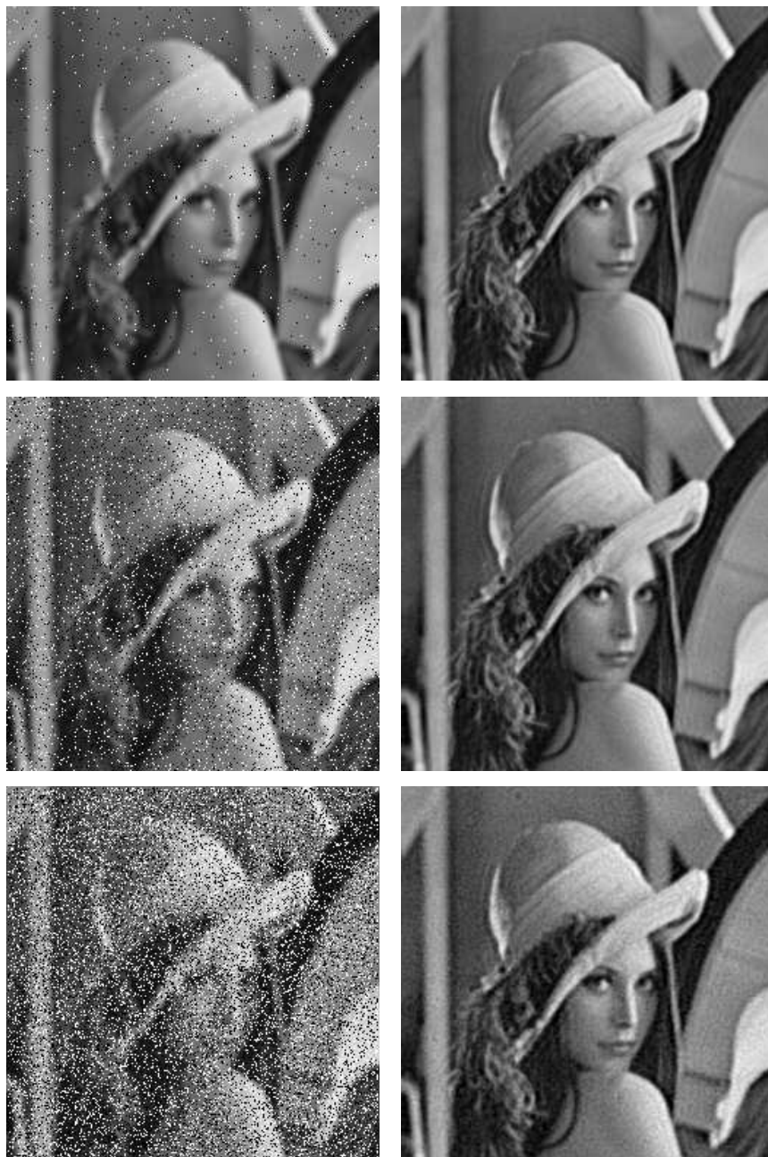
Fig. 4. Left column: The Lena image, blurred with a pill-box kernel of radius 3, and contaminated by salt and pepper noise. The noise densities are (top to bottom) 0.01, 0.1 and 0.3. Right column: The corresponding recovered images.
