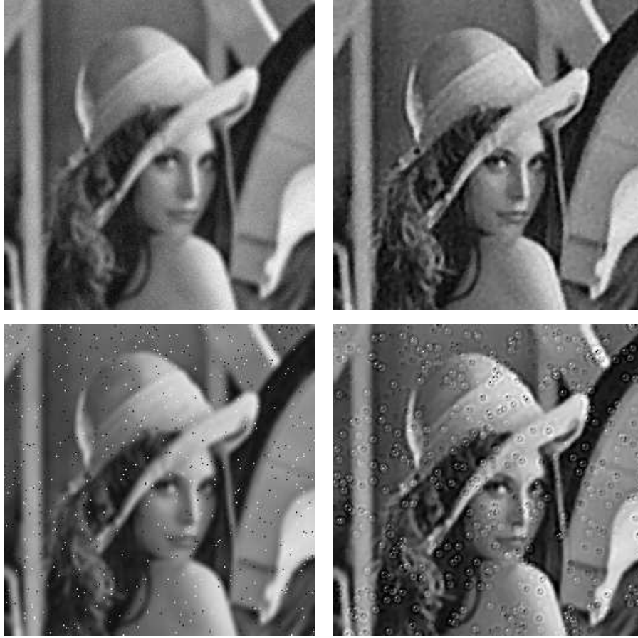
Fig. 1. Current image deblurring algorithms fail in the presence of salt and pepper noise. Top-left: Blurred image with Gaussian noise. Top-right: Restoration using the method of [23]. Bottom-left: Blurred image with salt and pepper noise. Bottom-right: Restoration using the method of [23].
