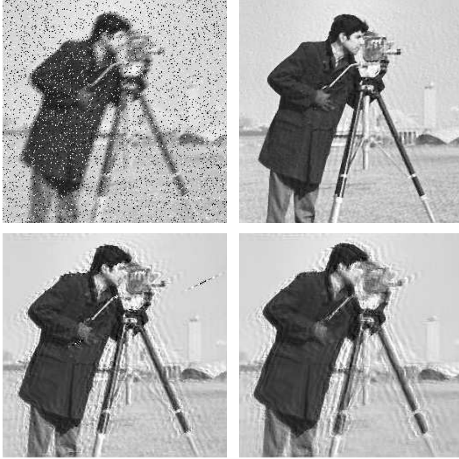
Fig. 5. The case of motion blur. Top-left: Blurred and noisy image. Top-right: Restoration using the proposed method. Bottom-left: The outcome of 3 \times 3 median filtering followed by Lucy-Richardson restoration (Matlab: deconvlucy ). Bottom-right: The outcome of 5 \times 5 median filtering followed by Lucy-Richardson restoration.
