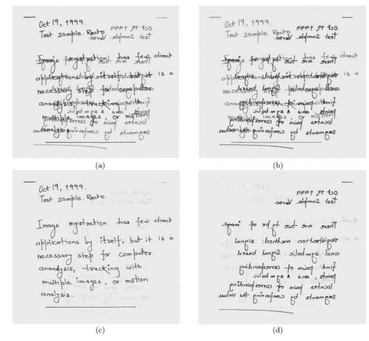
Fig. 1 Text separation with symmetric orthogonalization. a Recto of a real-fake manuscript showing bleed-through (from http://www.site.uottawa.ca/redubois/documents). b Flipped verso of the same manuscript. c First symmetric orthogonalization output. d Second symmetric orthogonalization output
