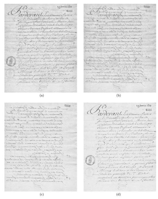
Fig. 3 Text separation by symmetric orthogonalization. a Recto of a real ancient document showing bleed-through (from http://www.site.uottawa.ca/redubois/documents). b Flipped verso of the same document. c First symmetric orthogonalization output. d Second symmetric orthogonalization output
